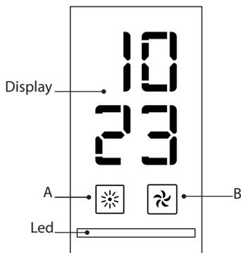
A.Light ON/OFF key: press this key to switch on or off the hood lights.
